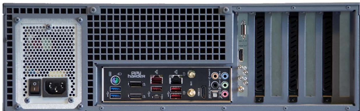
Figure 11: RTM 4K Back Panel (Supplied with five SMB to BNC conversion cables for 4 inputs and one reference. Optional uncompressed IP card shown in photo.) Model: RTM-S8085 (8 TB storage model)
