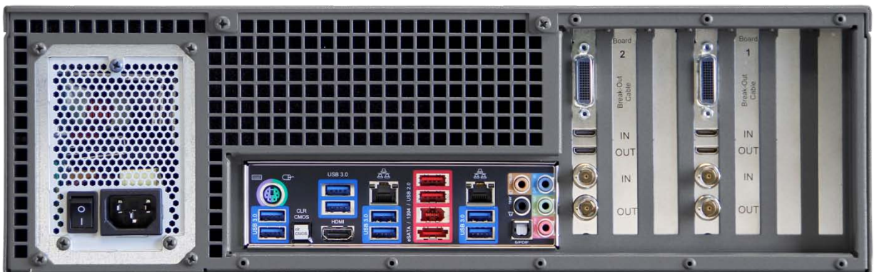
Figure 4: RTM 3G Portable Back Panel (supplied with SMB to BNC, mini HDMI and also supplied with analog breakout cables for playback)
